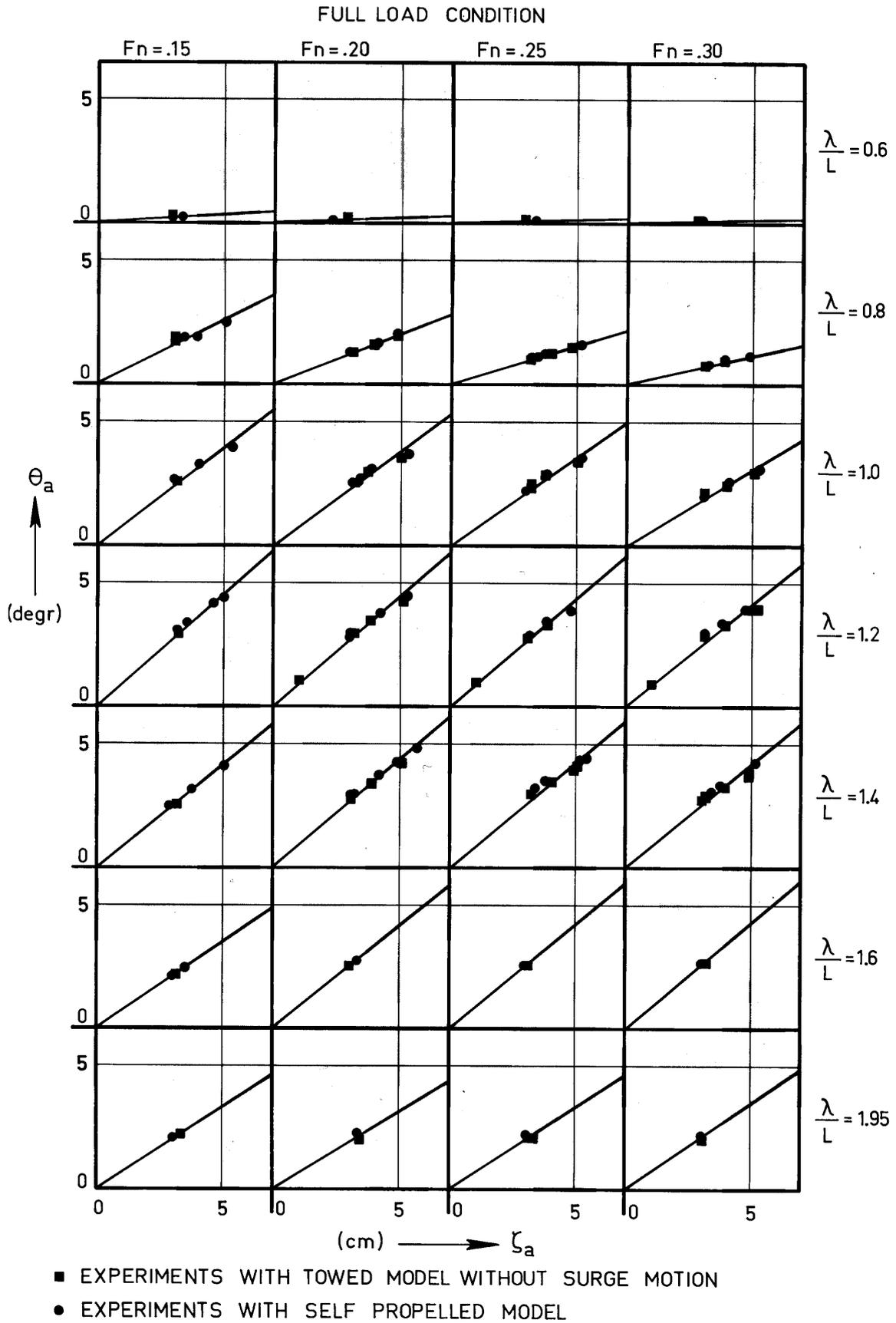
Figure 8 Relation between Pitch and Wave Amplitude
