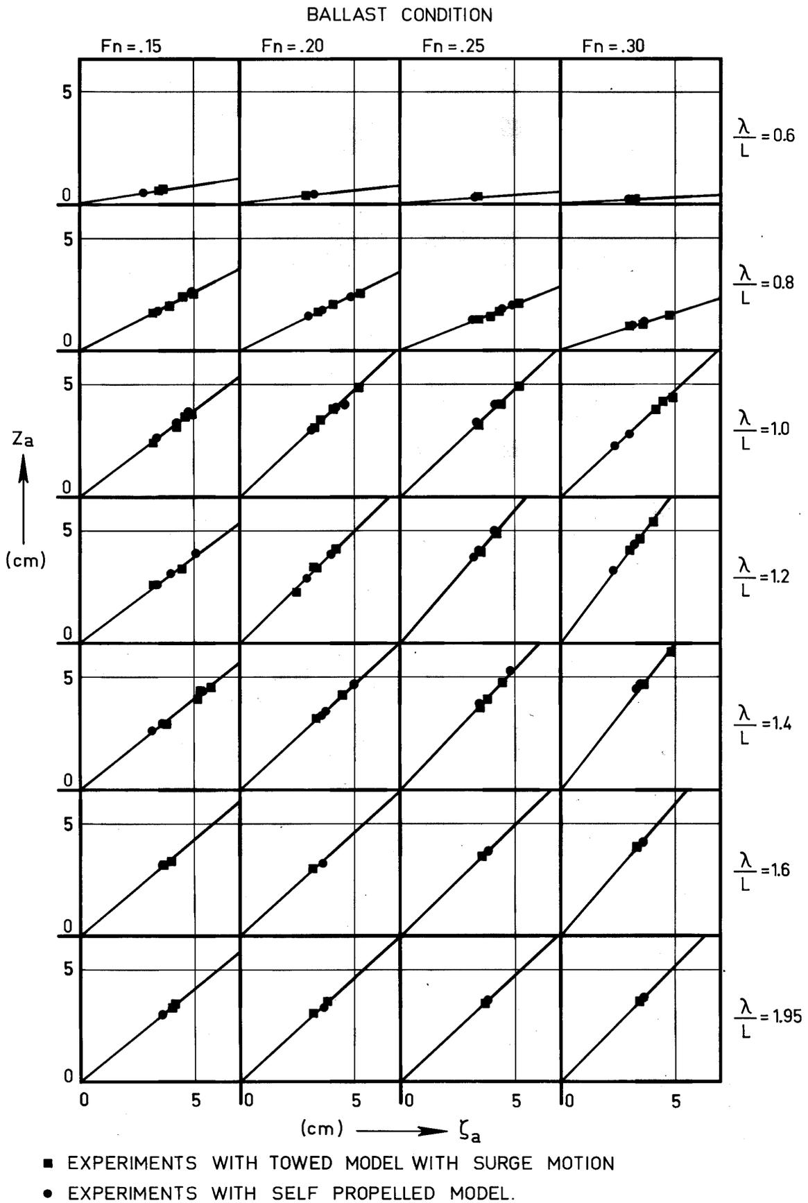
Figure 5 Relation between Heave and Wave Amplitude
