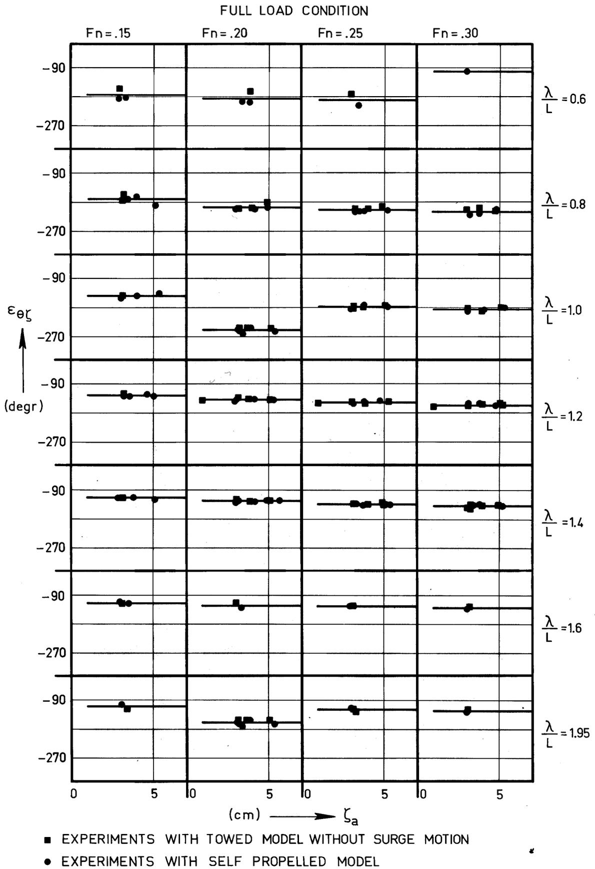
Figure 10 Relation between Phase Lag of Pitch and Wave and Wave Amplitude (Full Load Condition)
