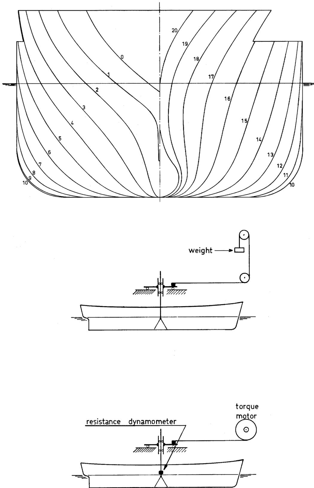
Figure 2 Body Plan and Arrangement for Resistance Tests
