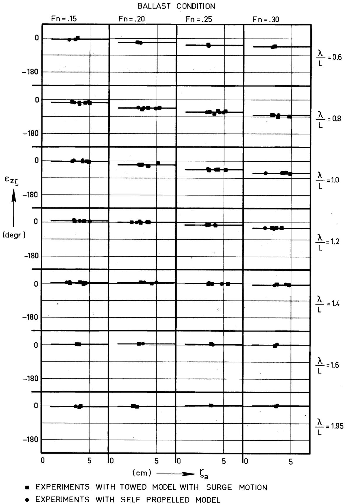
Figure 7 Relation between Phase Lag of Heave and Wave and Wave Amplitude (Ballast Condition)
