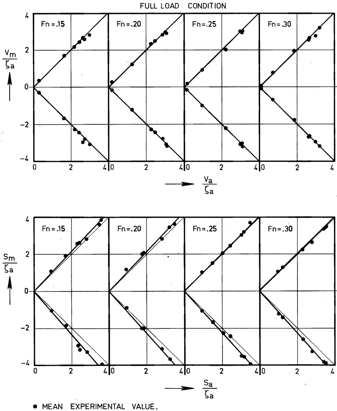
Figure 18 Relation between Measured Extreme Values of Absolute and Relative Motion and Motion Amplitude Calculated from Heave, Pitch and Wave (Full Load Condition, Station 20)
