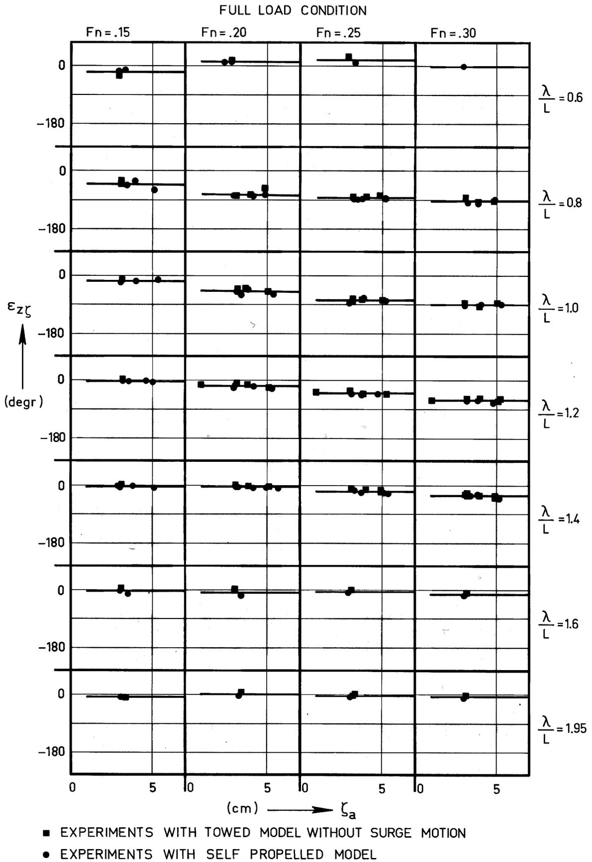
Figure 6 Relation between Phase Lag of Heave and Wave and Wave Amplitude (Full Load Condition)
