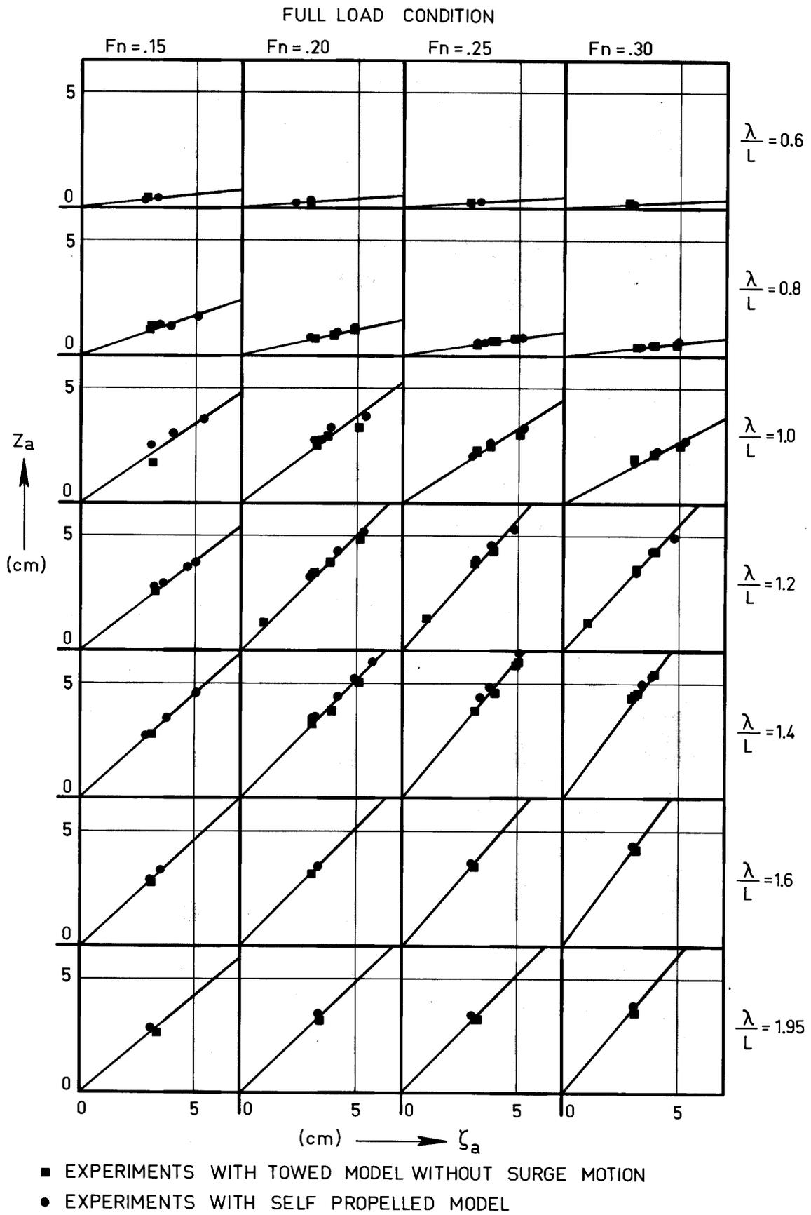
Figure 4 Relation between Heave and wave Amplitude
