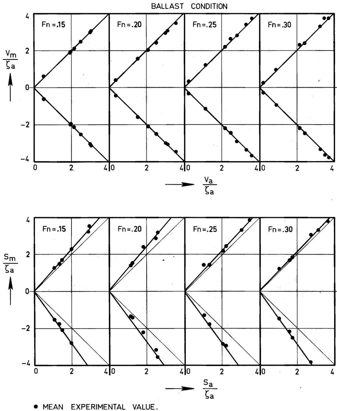
Figure 19 Relation between Measured Extreme Values of Absolute and Relative Motion and Motion Amplitude Calculated from Heave, Pitch and Wave (Ballast Condition, Station 18)
