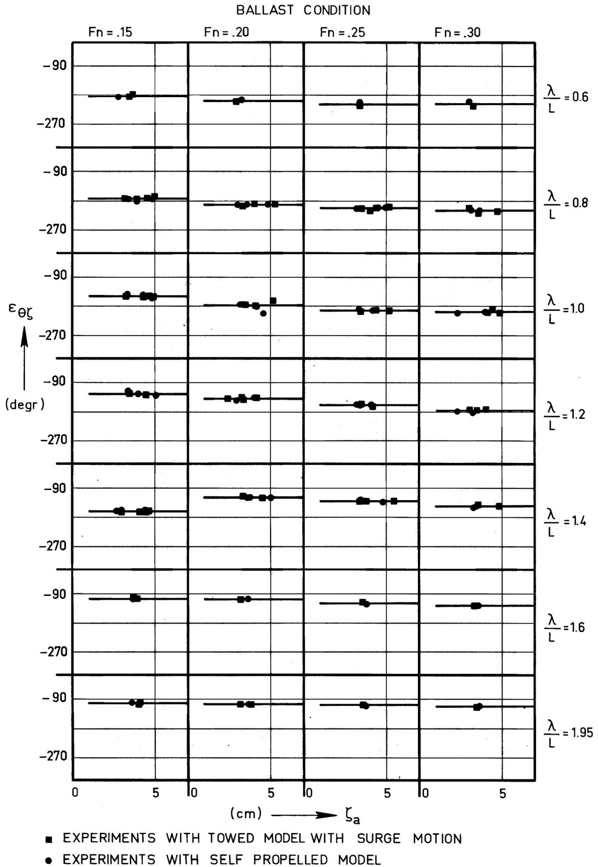
Figure 11 Relation between Phase Lag of Heave and Wave and Wave Amplitude (Ballast Condition)
