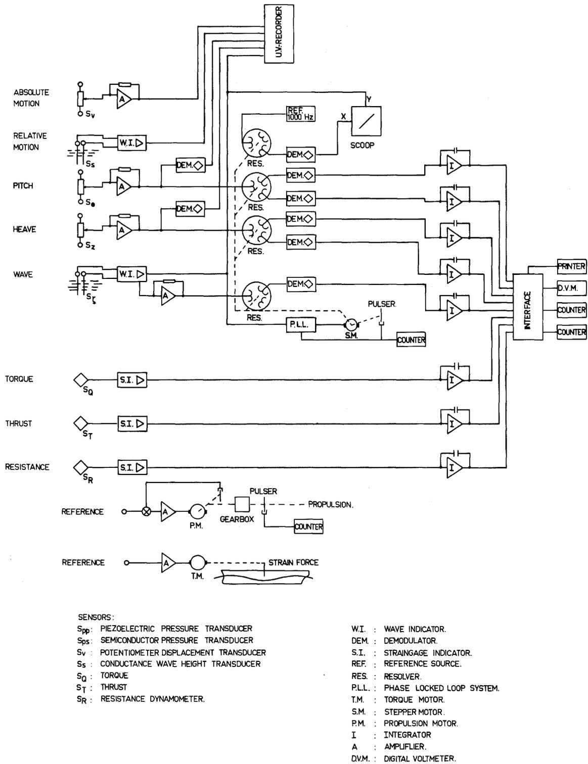
Figure 3 Scheme of Measuring System
