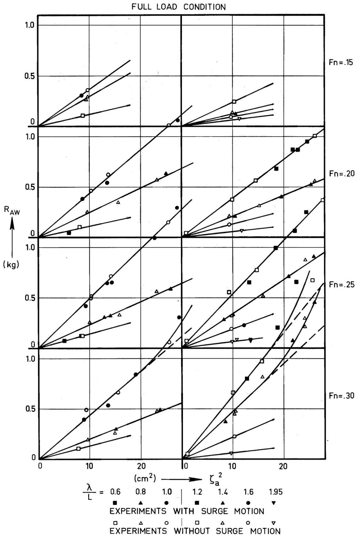
Figure 22 Relation between Added Resistance and Wave Amplitude Squared (Full Load Condition)
