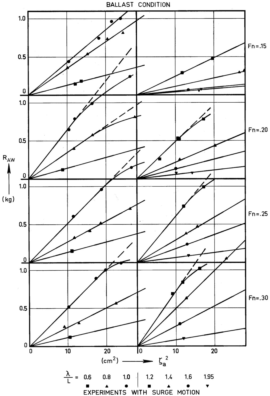
Figure 23 Relation between Added Resistance and Wave Amplitude Squared (Ballast Condition)
