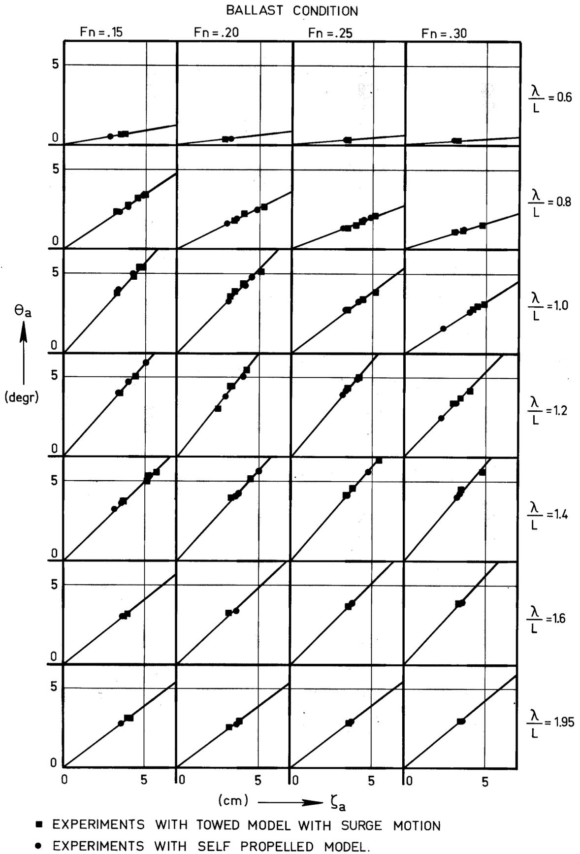
Figure 9 Relation between Pitch and Wave Amplitude
