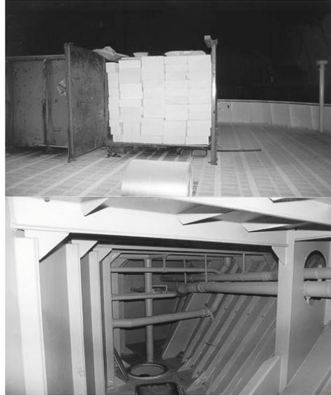
Figure 5 EPS foam blocks as used in ferry SIER (top), wing tank i.w.o. ER after 5 years of foam stowage (bottom).
