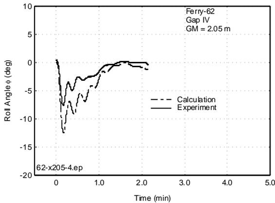
Figure 38 Measured and Calculated Roll of Ferry-62 for  $GM = 2.05$  m
