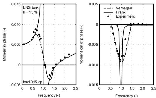
Figure 9 Roll Moments of an LNG Tank with 15 % Filling Level
