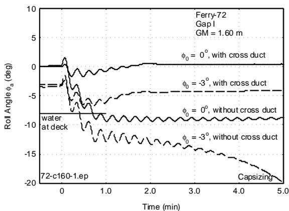
Figure 33 Influence of Cross Duct on Capsizing of Ferry-72
