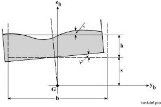
Figure 1 Axis system and Notations
