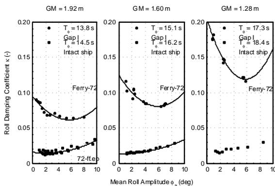
Figure 30 Roll Damping of Ferry-72
