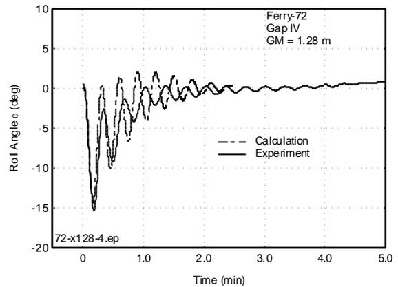
Figure 39 Measured and Calculated Roll of Ferry-72 for  $GM = 1.28$  m
