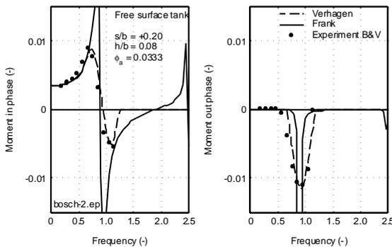
Figure 6 Roll Moments of a Free Surface Tank with Bottom above G
