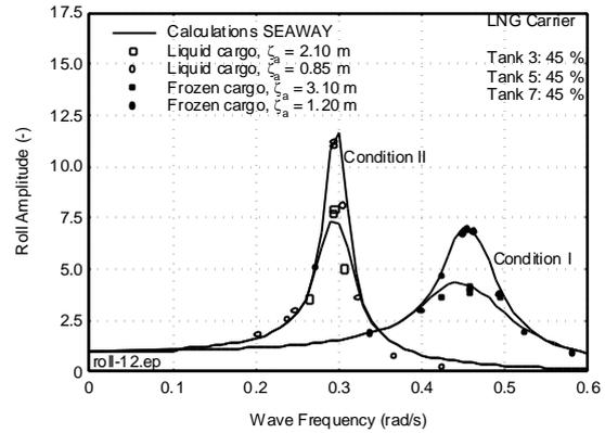
Figure 17 Roll Motions of LNG Carrier, Conditions I and II
