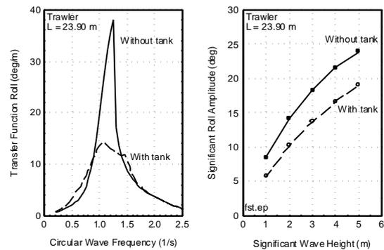
Figure 7 Effect of Free-Surface Anti-Roll Tank on Roll
