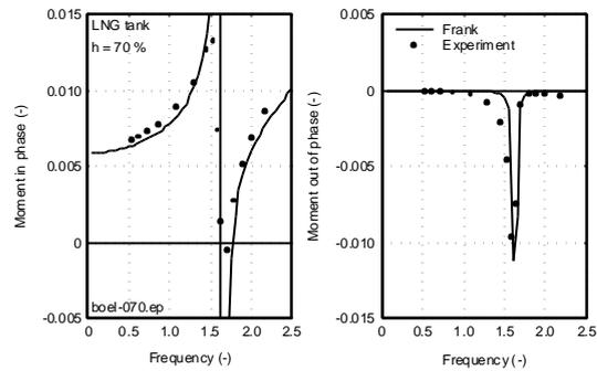
Figure 11 Roll Moments of an LNG Tank with 70 % Filling Level
