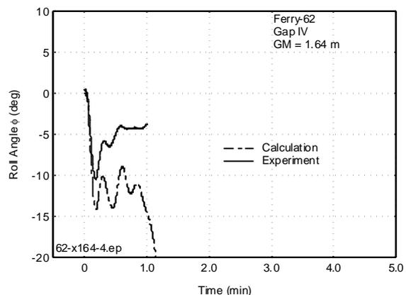
Figure 37 Measured and Calculated Roll of Ferry-62 for  $GM = 1.64$  m
