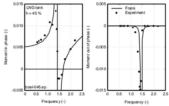
Figure 10 Roll Moments of an LNG Tank with 45 % Filling Level
