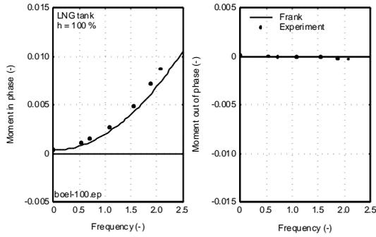
Figure 14 Roll Moments of an LNG Tank with 100 % Filling Level
