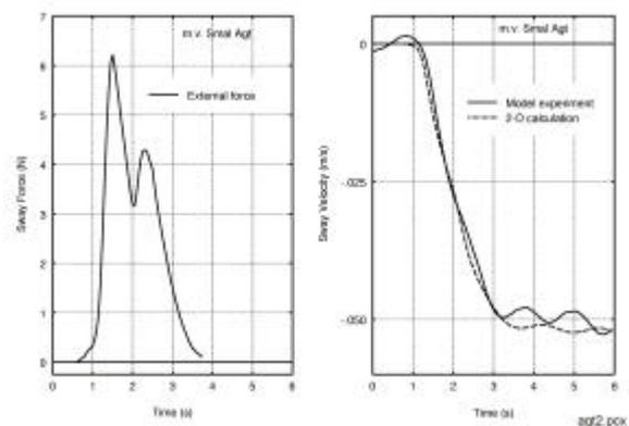
Figure 20 External Impulse and Resulting Motions
