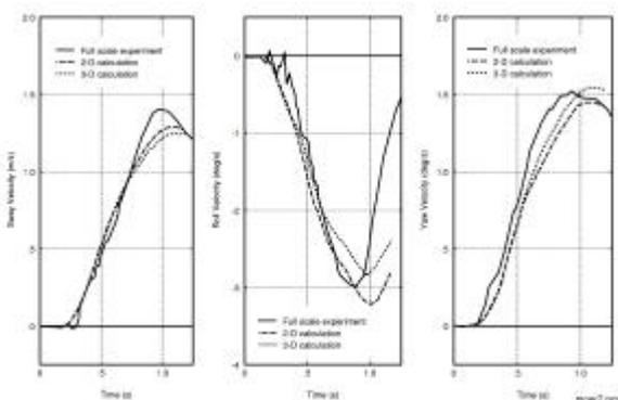
Figure 22 Velocities during a Ship Collision
