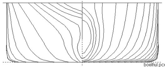
Figure 15 Body Plan of LNG Carrier
