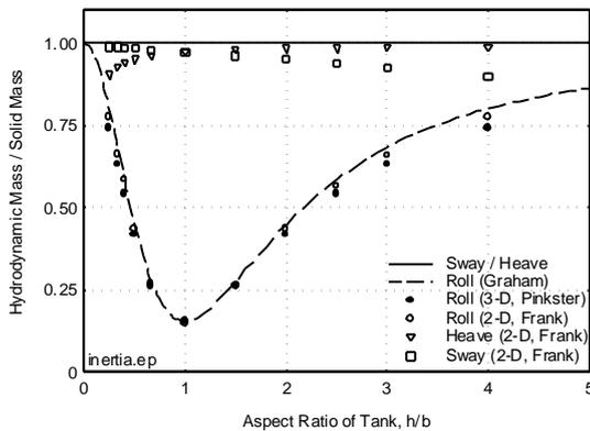
Figure 3 Moment of Inertia of a Fully Filled Tank
