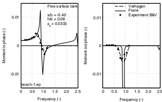
Figure 5 Roll Moments of a Free Surface Tank with Bottom below G
