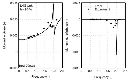
Figure 12 Roll Moments of an LNG Tank with 90 % Filling Level
