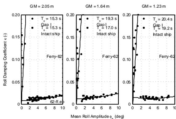
Figure 26 Roll Damping of Ferry-62
