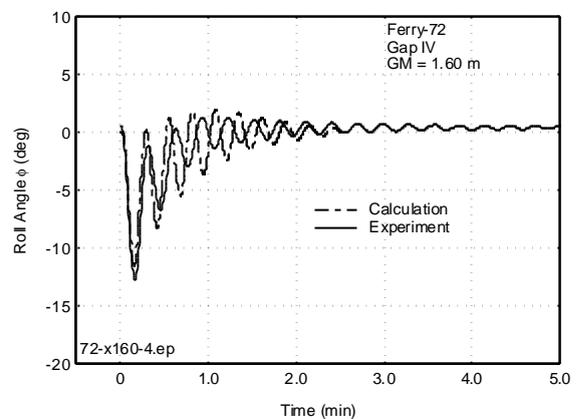
Figure 40 Measured and Calculated Roll of Ferry-72 for  $GM = 1.60$  m
