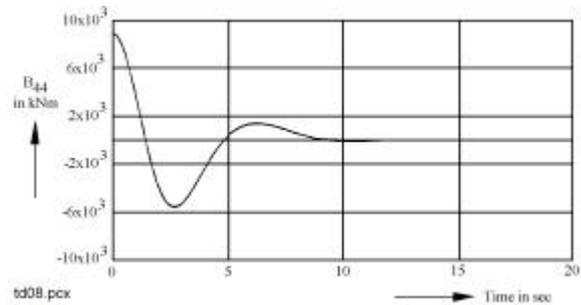
Figure 19 Retardation Function for Roll
