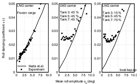
Figure 16 Roll Damping Coefficients
