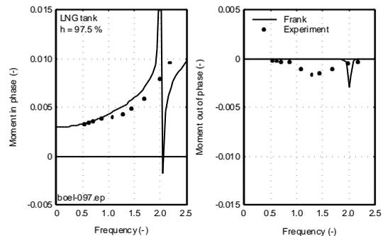
Figure 13 Roll Moments of an LNG Tank with 97.5 % Filling Level
