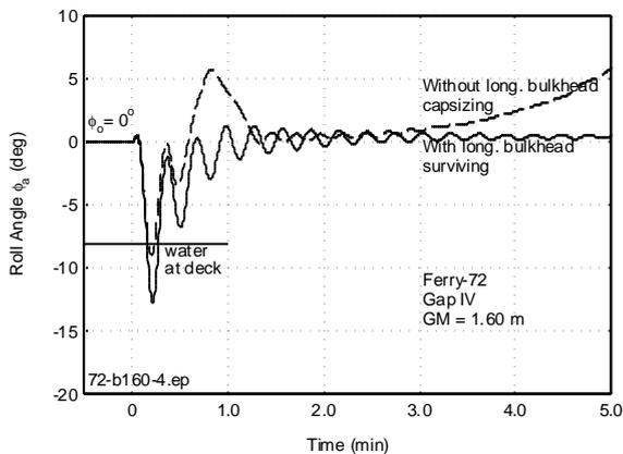
Figure 32 Influence of Longitudinal Bulkhead on Capsizing of Ferry-72
