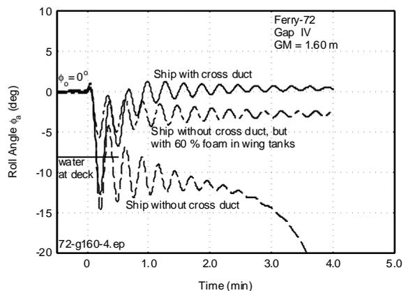
Figure 34 Influence of Permeability of Wing Tank on Capsizing of Ferry-72
