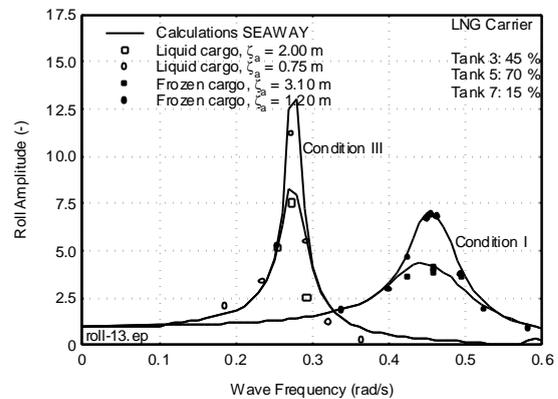
Figure 18 Roll Motions of LNG Carrier, Conditions I and III
