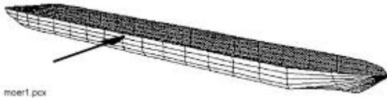
Figure 21 Under Water Portion of Rammed Ship
