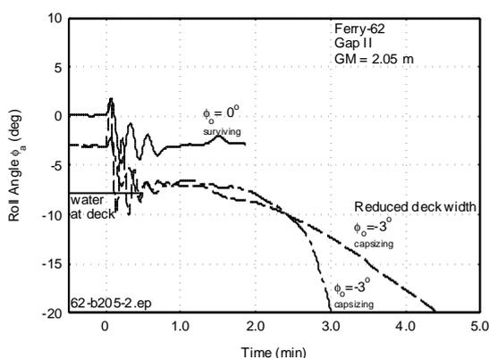
Figure 28 Influence of Reduced Deck Width on Capsizing of Ferry-62
