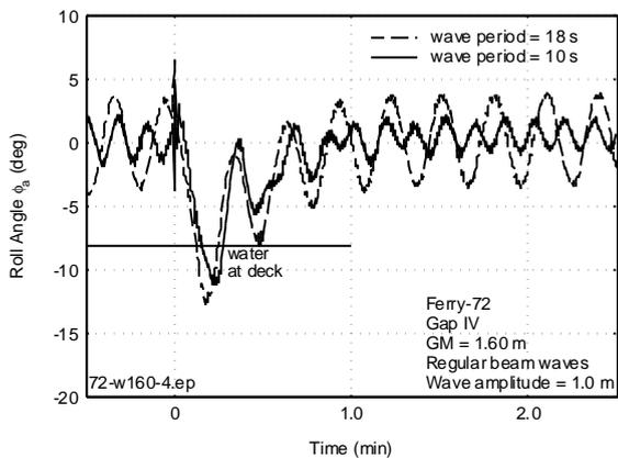
Figure 36 Influence of Regular Beam Waves on Capsizing of Ferry-72
